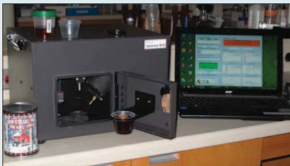
FIGURE 1. SpectrAcer prototype developed by Agriculture and Agri-Food Canada and Centre ACER for adulteration detection and quality control of maple syrup.
